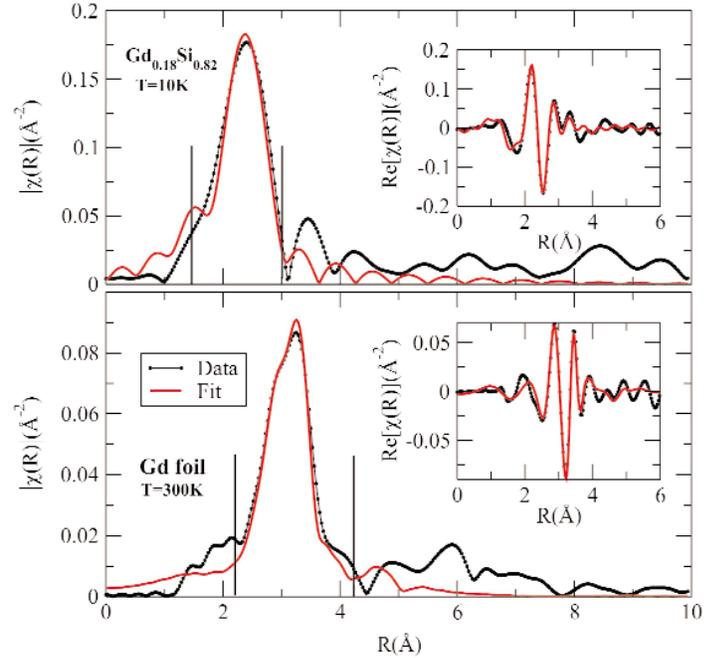
FIG. 1. Magnitude of the complex Fourier transform of the XAFS signal at the Gd  $L_3$  edge of a  $x=0.18$  sample (top) and for a Gd metal foil (bottom). The vertical lines show the region of real space fitted. The insets show the real part of the complex Fourier transform.
