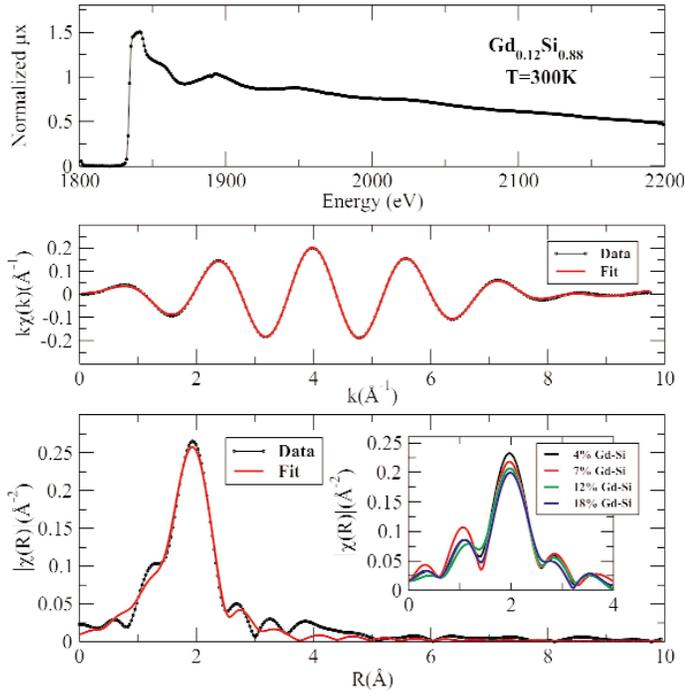
FIG. 2. Normalized absorption (top), first shell XAFS (middle), and real-space data and fits at the Si K-edge of a  $x=0.12$  sample. The inset in the lower panel show the reduction in first shell amplitude as the Gd concentration increases.
